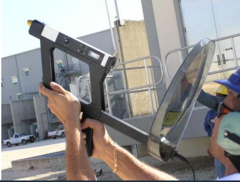
The PowerBeam 300 Was Designed To Test High Voltage Insulators And Transformers From A Safe Distance With A High Degree Of Accuracy.
